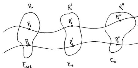
**Figura 2.3:** Evolución de un volumen de fluido mediante el flujo.  $P_1 = \gamma_{P_1}[0] = \mu_0[P_1]$ ,  $P_1' = \gamma_{P_1}[s] = \mu_s[P_1]$ ,  $P_1'' = \gamma_{P_1}[s+t] = \mu_{s+t}[P_1]$ ,  $P_2 = \gamma_{P_2}[0] = \mu_0[P_2]$ ,  $P_2' = \gamma_{P_2}[s] = \mu_s[P_2]$ ,  $P_2'' = \gamma_{P_2}[s+t] = \mu_{s+t}[P_2]$ .  $E_{s+t} \rightarrow E_t \rightarrow E_0$ .
